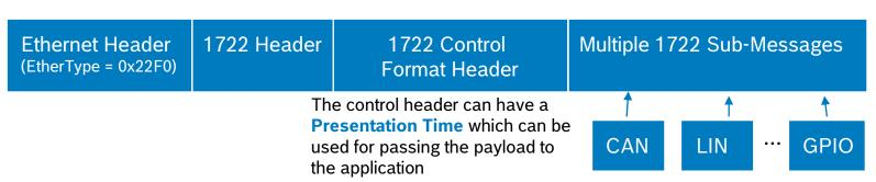
Each sub-message can have an **Acquisition Time** field which can be used for sensor fusion
