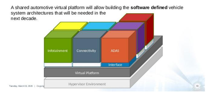
The outlook of a standard virtual platform may enable the necessary future flexibility and achievability of complex automotive systems.
