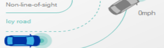
Blind curve hazard warning
