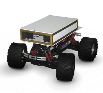
DNN-based self-driving robot Training data by human driver No hand-coded CV algorithms
