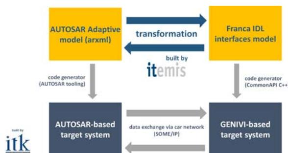
The ARA-to-Franca tool is implemented using the Xtend language, which is an extension of Java providing language features which ease the implementation of model-to-model transformations. It uses Artop (release 4.10) as an implementation of Adaptive AUTOSAR and Franca 0.13.0. Both are using the Eclipse Modeling Framework, which provides a common way of working with models.
