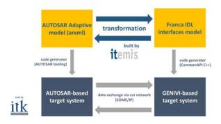
The ARA-to-Franca tool is implemented using the Xtend language, which is an extension of Java providing language features which ease the implementation of model-to-model transformations. It uses Artop (release 4.10) as an implementation of Adaptive AUTOSAR and Franca 0.13.0. Both are using the Eclipse Modeling Framework, which provides a common way of working with models.
