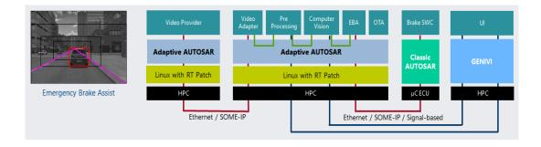
The common basis for communication between the ECUs is established using SOME/IP. However, on top of the protocol stack, different middleware such as CommonAPI and ARA::COM is used as binding to the applications.
