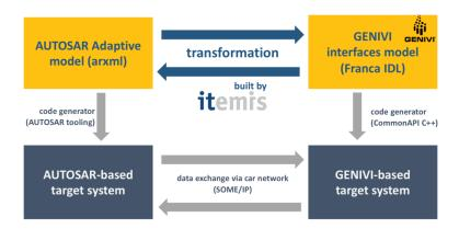
The ARA-to-Franca tool is implemented using the Xtend language, which is an extension of Java providing language features which ease the implementation of model-to-model transformations. It uses Artop (release 4.10) as an implementation of Adaptive AUTOSAR and Franca 0.13.0. Both are using the Eclipse Modeling Framework, which provides a common way of working with models.
