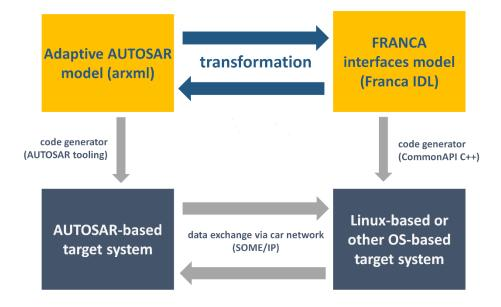
The ARA-to-Franca tool is implemented using the Xtend language, which is an extension of Java providing language features which ease the implementation of model-to-model transformations. It uses Artop (release 4.10) as an implementation of Adaptive AUTOSAR and Franca 0.13.0. Both are using the Eclipse Modeling Framework, which provides a common way of working with models.
