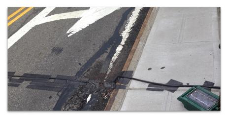
Cities currently collect traffic data by laying tubes on a road to record wheel passes. These studies typically collect data for 2 weeks before raw data is processed and ready for use.
