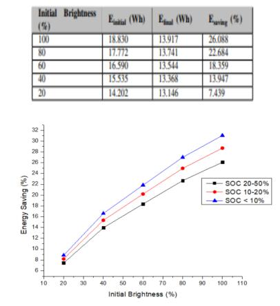
Observation: At high display brightness, if optimization is applied to minimize brightness, then maximum power savings achieved
